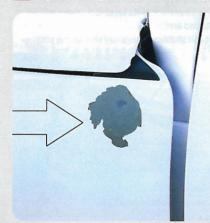
Paint and clearcoat flake is a common problem with late-model vehicles with waterborne two- and three-stage factory paints. As we understand it from seasoned body shop professionals, the problem is paint adhesion and the sun's harmful UV rays. When waterborne paint entered factory production in the late '80s and early '90s, paint flake immediately ensued. Paint technology has improved considerably in the years since.
