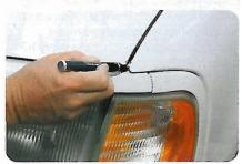
Paint Pen is a three-step process including primer, basecoat and clearcoat. Gently sand the scratch/nick, carefully apply primer to the damage, lay down basecoat, and seal the deal with clearcoat. Think of Paint Pen as a paint job for tiny damage.
