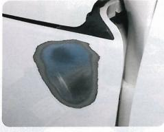
Surfaces are wiped with the provided tack cloth to eliminate any dust. Don't touch surfaces, Skin oil will attract dust and adversely affect paint adhesion.
