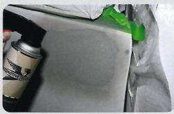
Using broad and even passes, apply Automotive Touchup sandable primer. It's suggested you use an acid-etch primer over bare steel first before laying down the sandable primer. We will get different opinions on this one, but self-etching primer-sealer etches and protects raw steel before the application of sandable primer. Sandable primer is the working primer you wet sand to perfection before the adding the basecoat.
