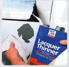
Automotive Touchup suggests beginning preparation with 180-320grit sandpaper to remove rust, scratches and damaged paint. Where it gets challenging with damaged and flaking paint is wondering where
