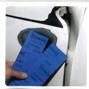
Automotive Touchup provides you with high quality 180, 320, 600, 1000 and 1500-grit abrasives. Depending upon the area you have to work with, this should be plenty of paper. Initial cutting needs to be performed with 180-grit paper. When you transition to 320- and 600-grit paper, it should be done wet using water as a lubricant. For best results, sand surfaces diagonally in all directions to achieve a smooth, feathered edge.
