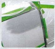
This is our completely primed repair area ready for wet sanding and the first layer of basecoat.
