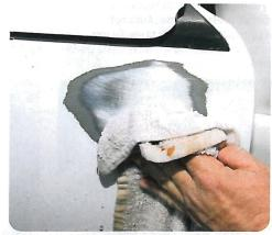
Once wet sanding is complete, wash down surfaces with soapy water then lacquer thinner to completely dry surfaces. Finish with a tack cloth to capture all dust and debris.
