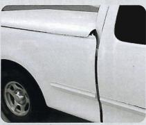
You can imagine our amazement when the job was finished, body shop quality with body basics from Automotive Touchup. Once the clearcoat was wet-sanded with 1500, it was time for a rubout with rubbing compound of the appropriate grit. Rubbing compound is available from Automotive Touchup.
