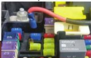
The wiring harness and fuse block needs to be run to a keyed 12-volt source. The main fuse panel for the Dodge is under the hood. A small hole needs to be drilled into the side of the fuse box and a suitable fuse that turns off with the key needs to be found. These types of fuses have an exposed pin on top of each spade so you can just touch the top of the fuse with a test light to find a fuse that turns off when the key is turned off. Keep in mind many trucks today have parking courtesy light that stay on for a few seconds after the key gets turned off. The connector hooks around the fuse and it gets plugged back into the fuse panel and a spade connector is used to attach the compressor.
