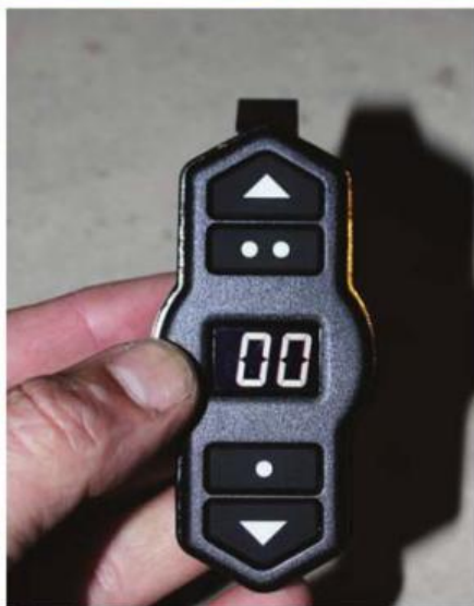
The wireless controller needs to have a couple batteries install and the arrows increase and decrease pressure to the air bags.
