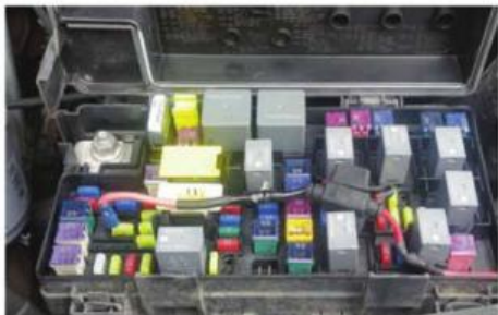
The wiring harness and fuse block needs to be run to a keyed 12-volt source. The main fuse panel for the Dodge is under the hood. A small hole needs to be drilled into the side of the fuse box and a suitable fuse that turns off with the key needs to be found. These types of fuses have an exposed pin on top of each spade so you can just touch the top of the fuse with a test light to find a fuse that turns off when the key is turned off. Keep in mind many trucks today have parking courtesy light that stay on for a few seconds after the key gets turned off. The connector hooks around the fuse and it gets plugged back into the fuse panel and a spade connector is used to attach the compressor.
