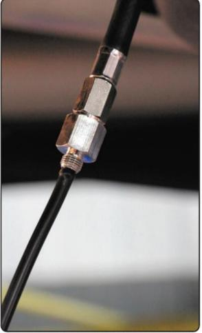
12 Next, a section of the supplied ¼-inch DOT approved air line was cut to length and attached to the compressor leader hose for the manifold filter. To get the hardy line over the barb, it was warmed slightly using a heat gun.
