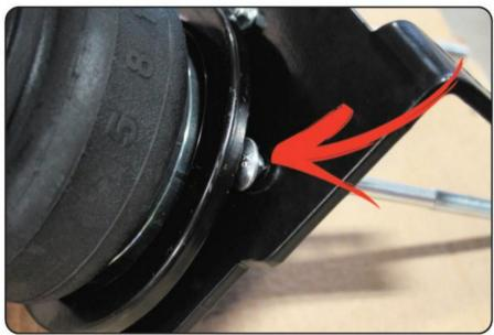
4 It's important to note that prior to the air spring being attached to the lower main bracket, Flynn had to determine which supplied 10-inch long carriage bolt went into its respective hole to clear the roll plate (the bottom support for what the air spring is seated in). Otherwise there won't be room later, as you can see here.
