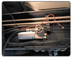
10 The compact size of the heavy-duty air compressor Air Lift provides makes finding a spot to mount it much easier than with other air spring kits on the market. Flynn chose to mount the air compressor along the frame rail directly in front of the fuel tank, which called for four 7/32-inch holes being drilled in the frame.
