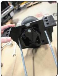
3 Chad Flynn of Flynn's Shop began the install by piecing together both air spring and bracket assemblies. First, the supplied roll pate was attached to the bottom of each air spring, and then the lower bracket cup was fastened to the lower main bracket (shown). The lower bracket cup is what sits on the factory leaf spring block perch.
