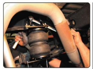
8 Because our '11 F-350 already had an aftermarket gooseneck hitch from B&W Installed, Flynn did not need to use the supplied hardware to connect the passenger side upper brace to the frame. Instead, the %-inch frame rail hardware from the B&W hitch was reused, while the remaining hardware supplied by Air Lift bolted the upper brace to the upper air spring assembly bracket.
