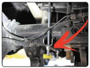
• The final piece in securing the air spring assemblies rested in the supplied clamp bars, which bolt to the bottom of the axle tube. Per Air Lift's instructions, the axle clamp bar bolts were torqued to the recommended 16 ft-lb. specification.
