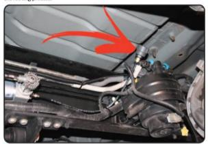
14 Given the positioning of the air compressor, Flynn was able to zip tie the compressor filter to the frame rail-mounted fuel filter assembly (arrow). Keeping the filter up and near the floorboard is important in keeping the compressor from ingesting any moisture.
