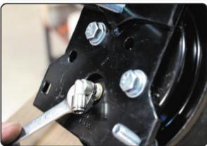
5 Next, the roll plate and upper bracket were installed on the topside of the air spring, followed by the 90-degree air fitting (swivel elbow, shown). The air fitting was first made hand-tight, and then tightened one and a half turns using a ½-inch wrench.
