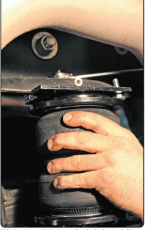
7 After the passenger side air spring assembly and top bracket spacer had been mocked up, Flynn tightened the nut on the bracket spacer. The primary link tying the air spring assembly to the frame rail would be the supplied passenger side upper brace.
