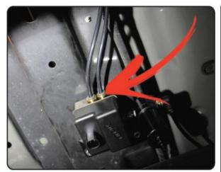
13 From there, the air lines running to each air spring were cut to the correct length and installed in the manifold (arrow). The air line on the left feeds air to the passenger side air spring, while the line on the right sends air to the driver side unit. All air lines were routed in and out of the frame rail and crossmembers at the rear of the truck to keep them safely out of harm's way, and zip ties were used throughout the routing process.
