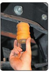
6 Once the air spring assemblies were built, Flynn turned his attention to the factory bump stops, which had to be discarded to install the air springs. Using penetrating oil and a 15mm socket, they were easily removed. Following that, the truck was placed on a 2-post truck lift to lower the rear axle away from the frame, relaxing the suspension.
