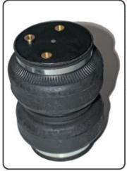
2 Built much like a tire, the Air Lift air springs feature durable, 2-ply fabric and cords for maximum strength and growth control. Upper and lower roll plates protect the springs from sharp edges and increase load carrying capacity by up to 10 percent. A closed-cell urethane foam jounce bumper also exists internally within the spring. This helps absorb shock, eliminates jarring on rough roads, and ultimately protects vehicles carrying heavy loads.
