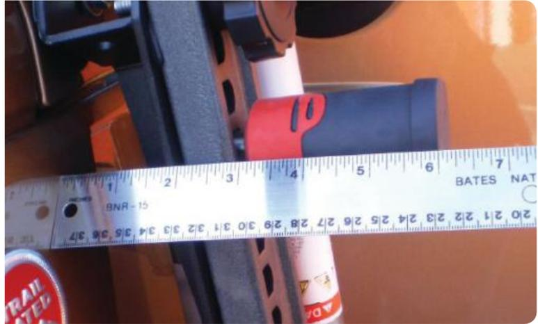
**With the lock in place, it extends 6" past the side of the Jeep. We'll likely remove it when on the trails to prevent hitting it.**
