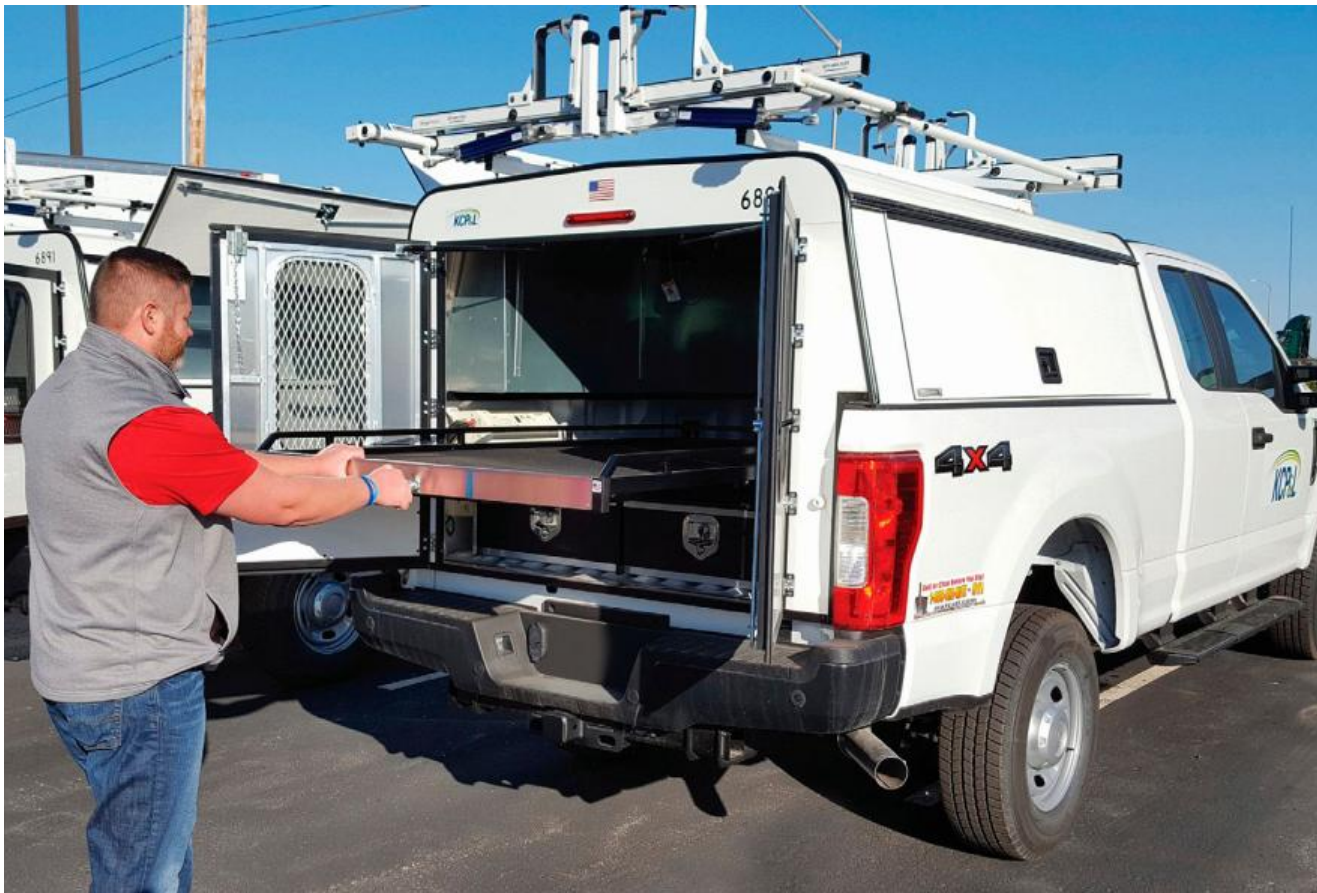
▲ LoadMaster sliding trays glide easily to bring heavy tools such as shop vacuums, power saws, toolboxes, and more to the individual, reducing the risk of potential injury.
