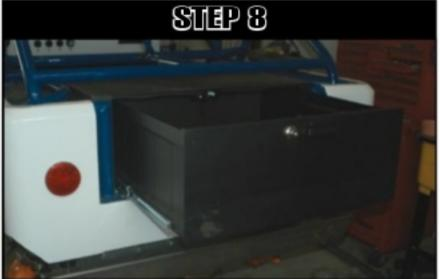
Another great option is the sliding cargo tray. I used this version in a previous Jeep, but could not in the TJ due to needing the battery in the back. The cargo box can hold cargo on top, the draw slides out and holds a ton of gear, and is easier to access stuff near the back.
