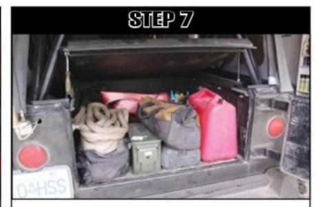
....Once swung open, the load tray can slide backwards and be lifted up for access to the back of the storage area, or removed completely if you need to carry taller gear. In my case, my tapered roll cage stops me from lifting the load tray right up, but it still slides out of the slots as normal.
