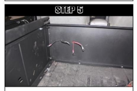
The rear wall of the storage unit attached to the sides with easy to remove twist knobs. The rear panel was drilled for the battery cables and grommets installed in each hole.
