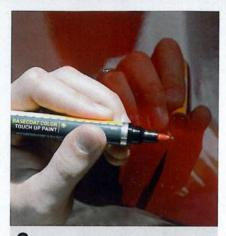
8 Fill out the area where the imperfection can be found. A steady hand is a benefit, so get a comfortable stable stance when applying. It shouldn't take much time.
