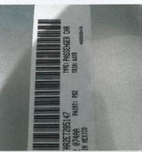
The first step to getting the right paint is finding the paint code, often on the door. Automotive Touchup offers a locator service on the website for various makes.
