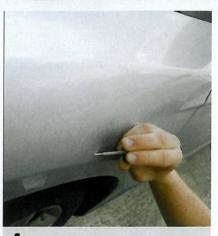
Lightly touch the area to be painted with the brush from the bottle. You should have tested the product on a glossy sheet of paper or metal can before starting. Be sure to blend the strokes and apply the product in an even coat.
