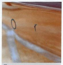
We've marked off some chip areas that are small enough to require only the paint pen. The pen can be used for areas that are the size of a pencil eraser or smaller.
