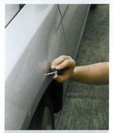
5 The two-ounce touchup bottle provides the basecoat, so a clearcoat will need to be added to finish the job.
